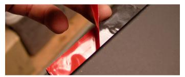
Figure 5.12b Peeling self-adhesive tape
