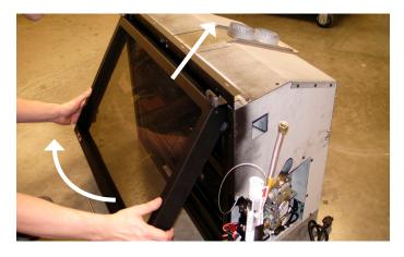
Check that the door retainers are properly engaged. If they are not the door relief system may not operate properly. This can cause a risk of injury or improper operation of the appliance.
