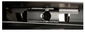
Engage door tool into door retainer. Pull door tool towards you and push downwards, disengaging the door retainer from the door.
