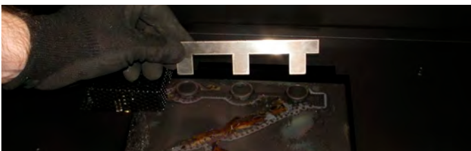
Figure 23.d Pushing the Rock Guard down into place.
