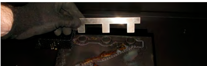
Figure 23.c Pushing the Rock Guard down into place.
