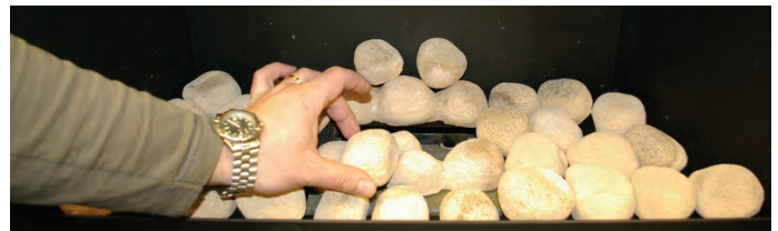
Figure 23.n Place the first Top faux Rock.
