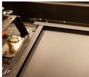
Figure 12.f Unscrewing brackets securing metal plate
