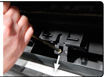
Figure 21.d Pull door latches
