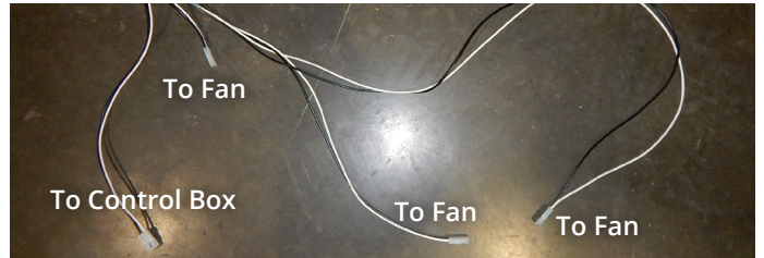
Figure 27.e Locate fan wiring harness
