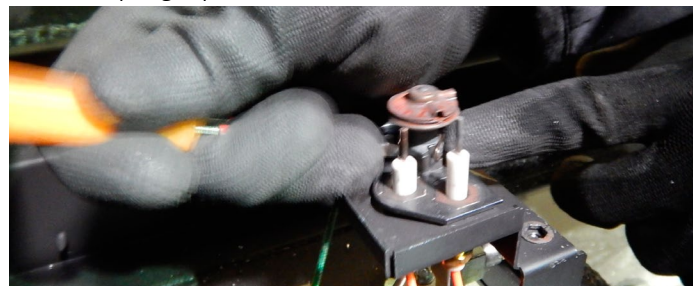
Figure 13.d Removing the spring clip
