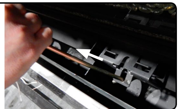
Figure 21.d Pull door latches
