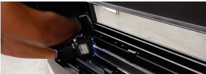
Figure 12.d Removing the Burner screws
