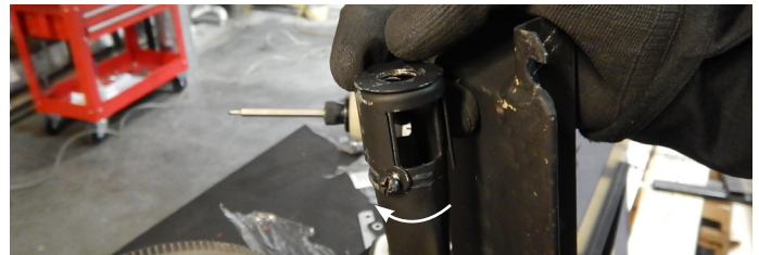
Figure 13.b Loosening the venturi
