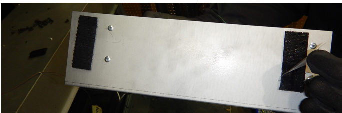
Figure 27.b prepare velcro strips
