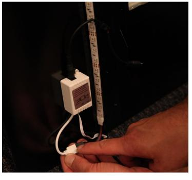
Remove adhesive cover from back of module and press against left side of the glass low enough so you can connect the RGB lights to and hang IR sensor just below the glass. Connect Adaptor wire to module and RGB lights to plug connecting the arrows together on 4 prong connector
