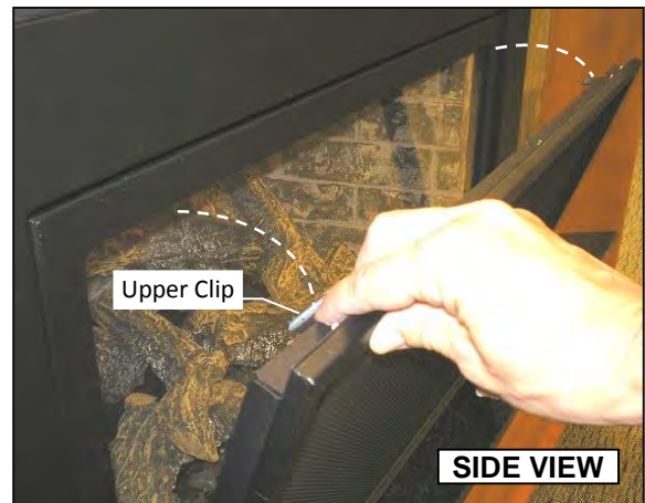
Press down and push upper clip under top glass door frame.
