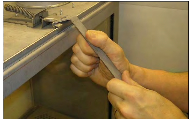
Step 4: Draw Latch forward with other hand.
