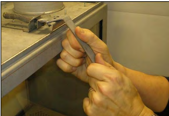
Step 5: Release Latch from Door.
