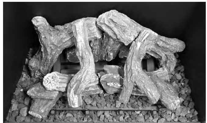
STEP 5: Place glowing embers on the front of the burner tube and ember plates. Place lava rock and vermiculite on the burner pan as shown. DO NOT PLACE LAVA ROCK AND VERMICULITE ON BURNER TUBE.
