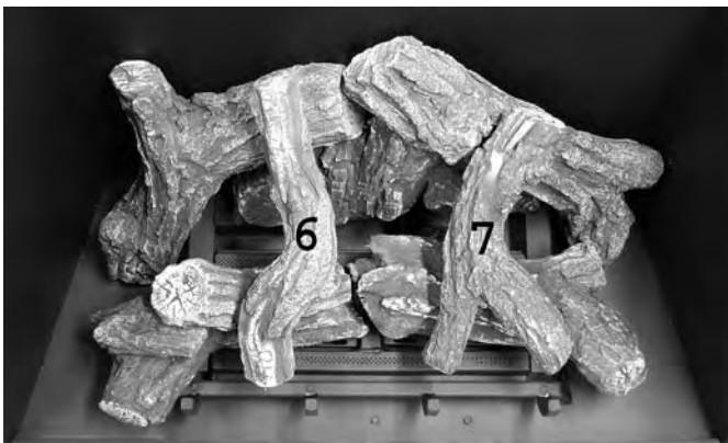
STEP 4: Locate the hole on the bottom of log #6. Place onto the mounting tab on log #2. Locate the 2 holes on the bottom of log #7. Place onto mounting tabs on log #5.
