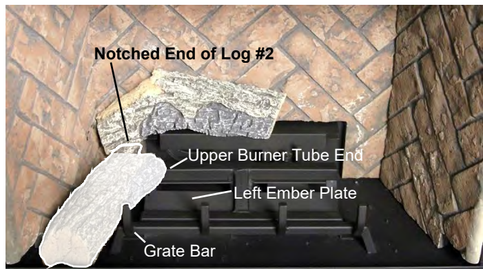
Step 2: Place Notched End of Log #2 onto Left Ember Plate and against Upper Burner Tube End. Next place Flattened Area of Log #2 onto Firebox Floor and against left side of Grate Bar.
