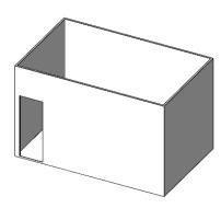
Walls on all sides (Minimum area of 96 square feet), but with no overhead cover and at least one permanent opening (doorway) at ground level.
