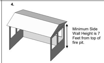
Within a partial enclosure that includes an overhead cover and three side walls, as long as <u>30 percent</u> or more of the horizontal periphery of the enclosure is permanently open.
