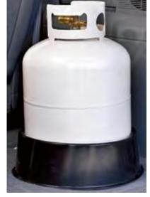
The above photo shows an example of an approved LP cylinder retention device.
