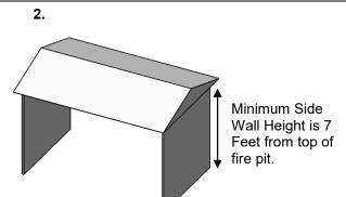
Within a partial enclosure that includes an overhead cover and no more than two side walls.
