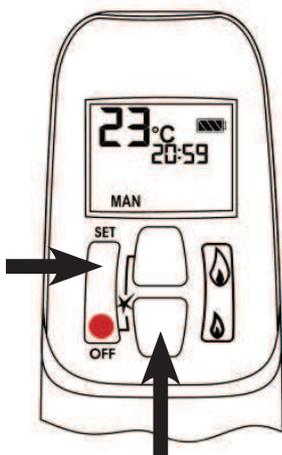
Turning off the “rear burner”:
