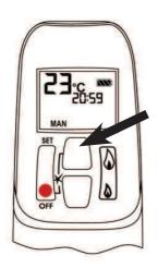
Press button (large flame) to increase the flame level and to turn on the burner from the stand-by position.
