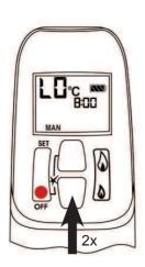
Pressing the (small flame) button twice automatically lowers the flames to the low position. (When this happens, the flames will first automatically go to maximum!) This is indicated by "LO" on the display.
