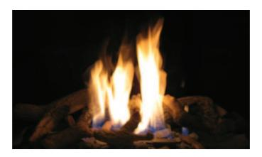
Figure 7: Burner flame appearance Centre Fire
