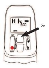
• Pressing the (large flame) button twice automatically increases the flames to the high position. This is indicated by "HI" on the display.
