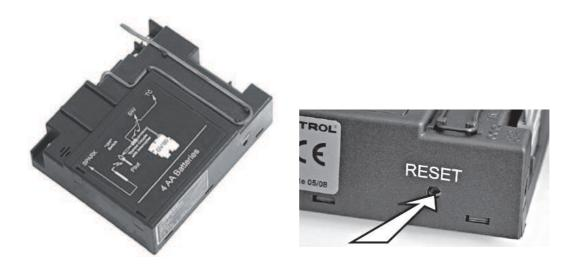
Figure 3: Receiver "RESET" button
