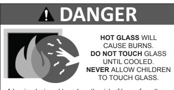
A barrier designed to reduce the risk of burns from the hot viewing glass is provided with this appliance and shall be installed for the protection of children and other at-risk individuals.
