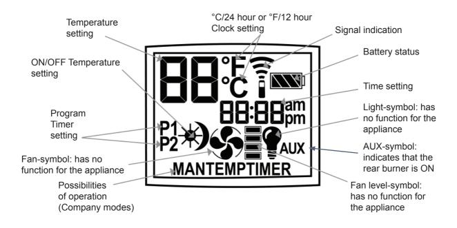
Figure 2: Display hand-held transmitter
